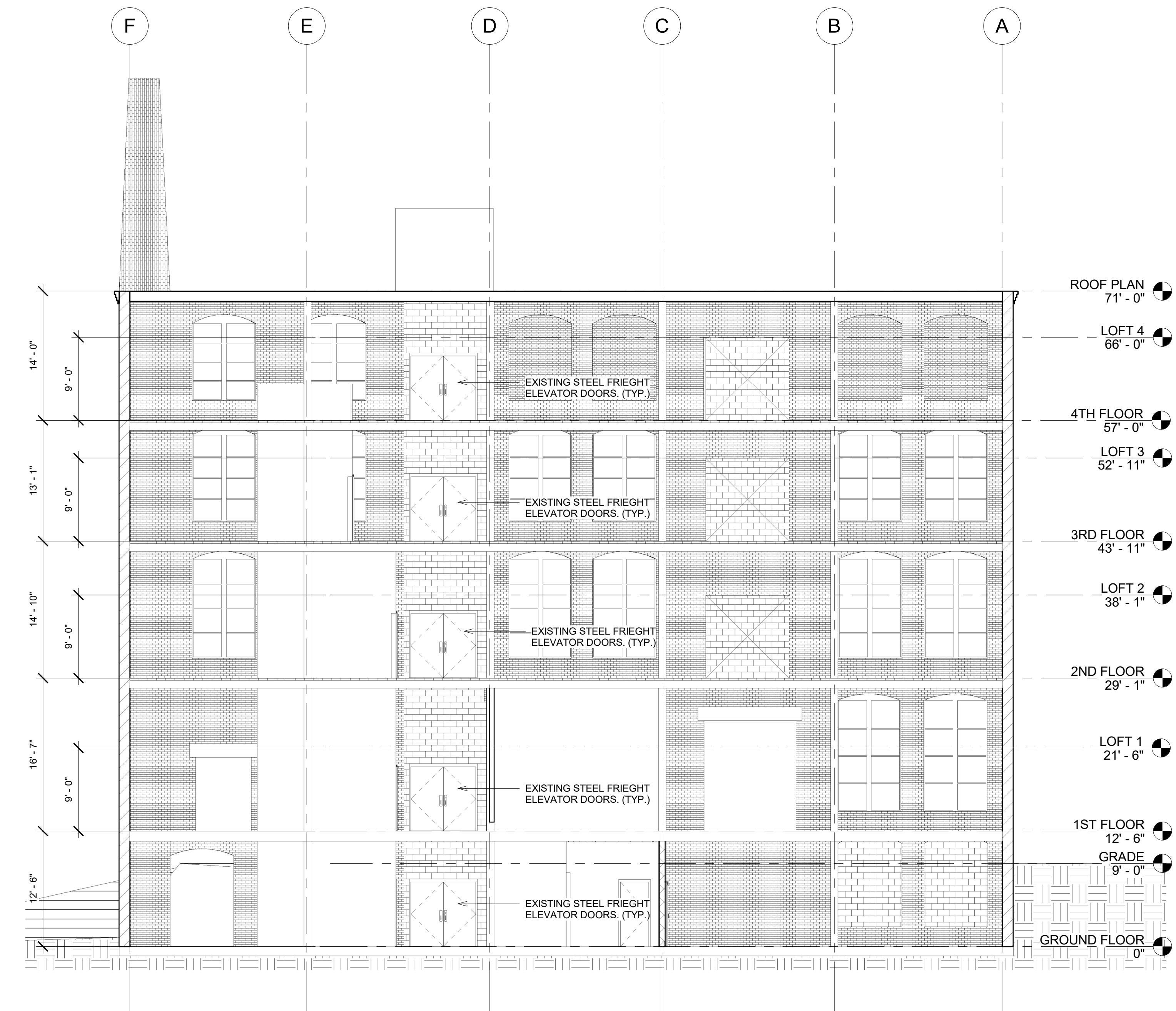
1 EXISTING BUILDING SECTION 1/8" = 1'-0"
