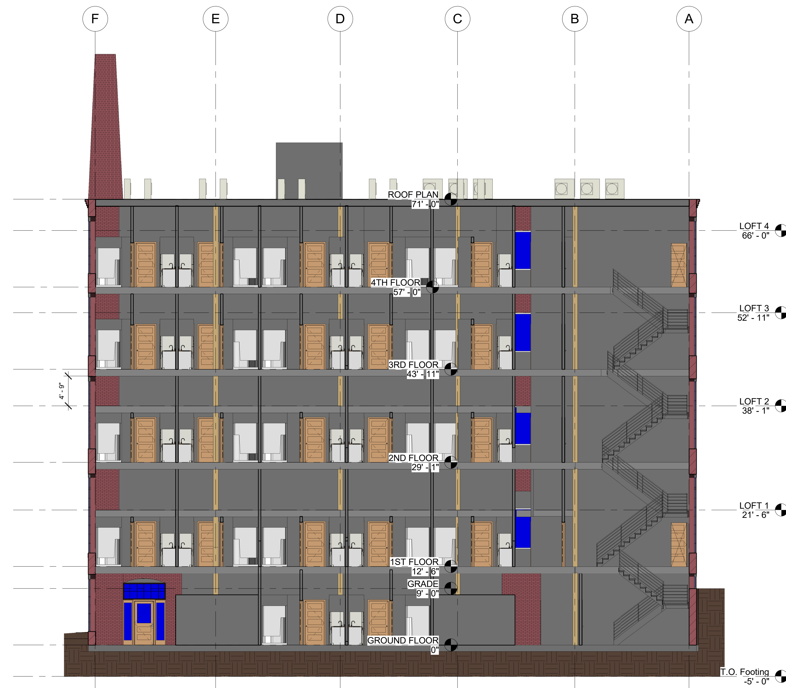
2 PROPOSED BUILDING SECTION 2 1/8" = 1'-0"
